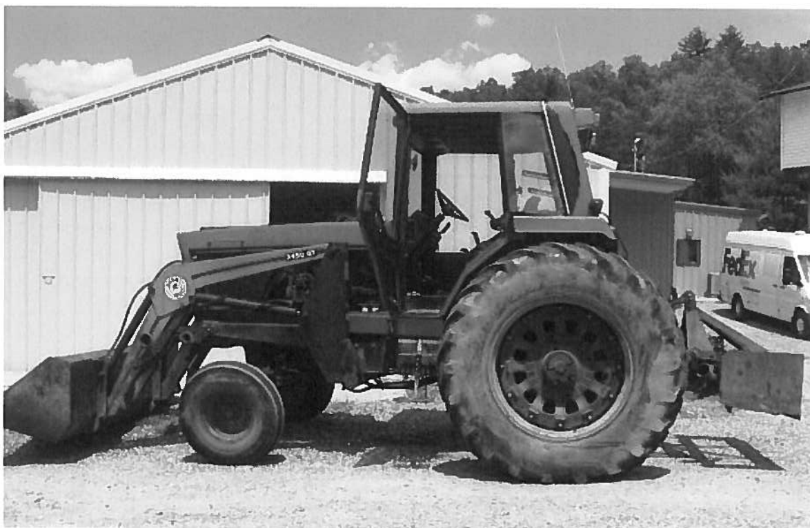
Figure 28. The cab compartment of this tractor is designed to serve as a ROPS. When operating around water, the cab door (which is only on the left side) should face away from the water so that the driver of an overturned and submerged tractor could escape through the
