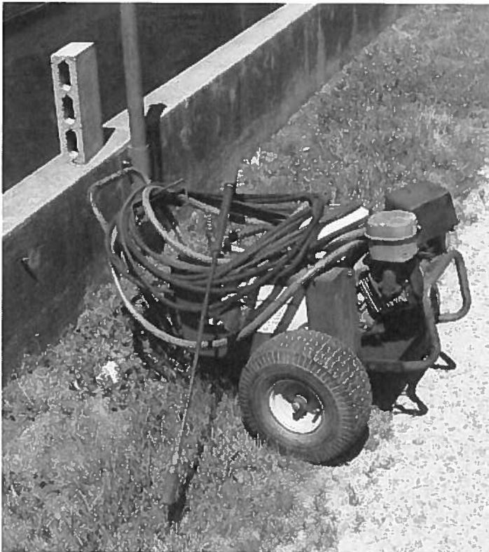
Figure 26. High-velocity water from pressure washers can cause skin injuries and bruises.
