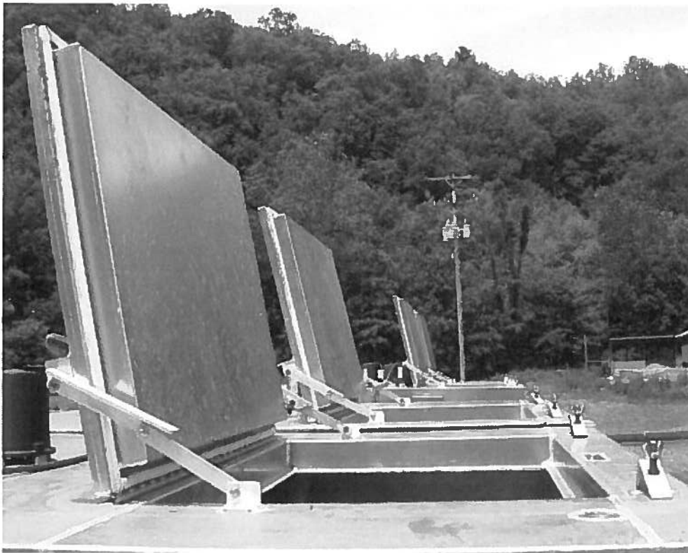
Figure 1. Locking hinges on live haul tank lids prevent the lids from falling on workers' hands.
