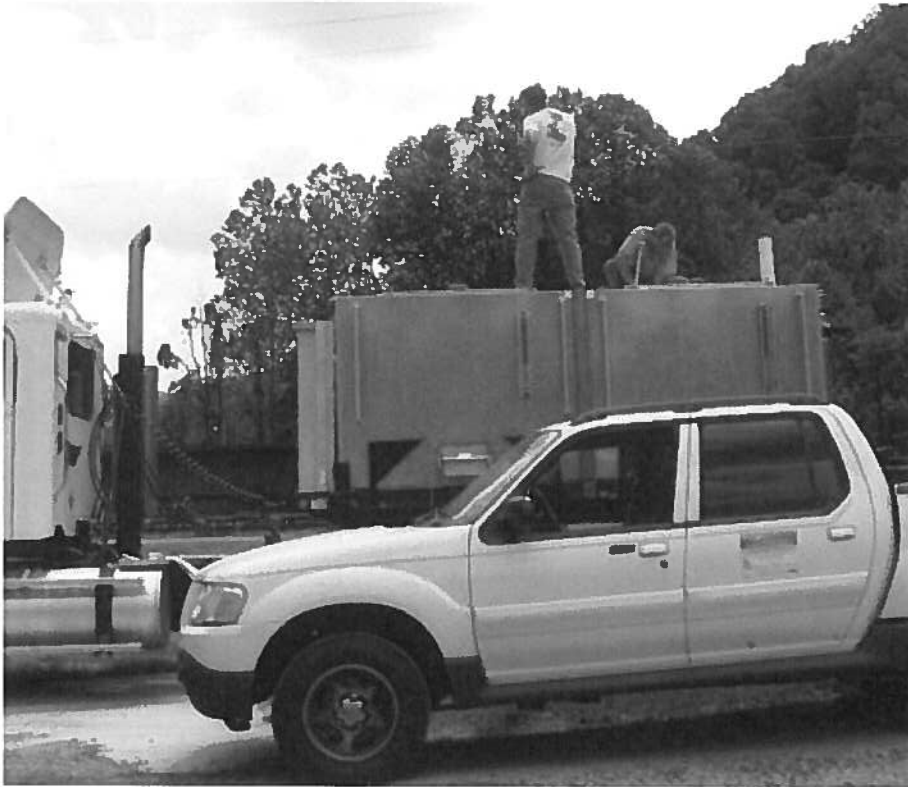
Figure 2. Falls from the top of live haul tanks are more likely when water, fish mucus, and ice are introduced. When loading is done inside a building, a safety harness can be suspended from the ceiling for workers to wear.
