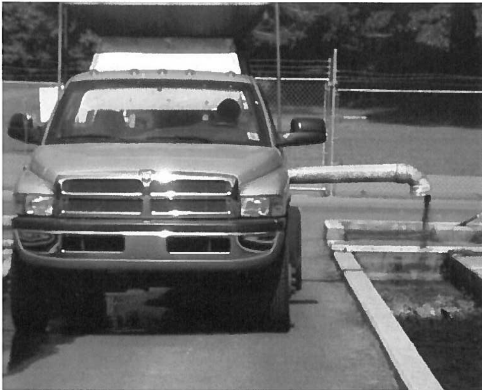
Figure 4. Feed trucks blow feed into raceways and alleviate the need to carry heavy feed bags
