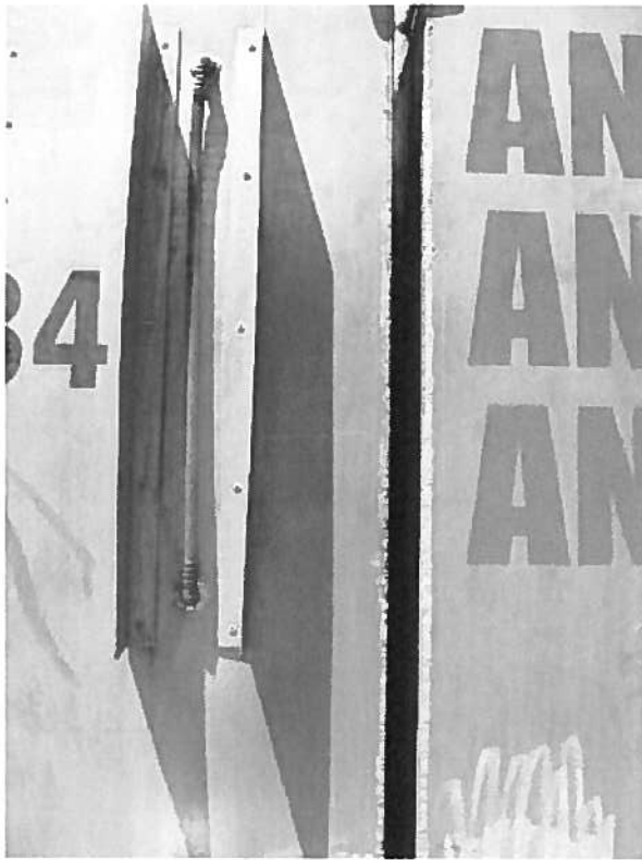
Figure 11. The clear plastic tube on the side of this live haul tank indicates the amount of water displaced when a load of trout is added to the tank.
